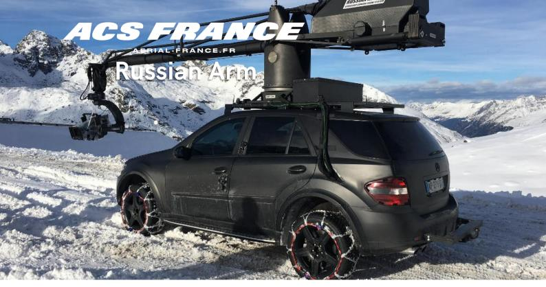
2 axis / Arm length from 4m to 7,60m / Pan 360° / Digital cinema / 150km/h
